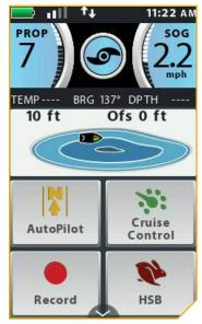
The Follow the Contour Active Band appears when the boat is navigating with Follow the Contour. The Contour being followed is 10 feet. The Offset is set to 0 feet.
