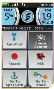
The Home Screen Buttons are Active and the Cruise Control button has been selected using the touch screen.
