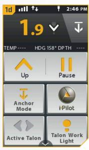
**NOTICE:** You do not need to press and hold the button to keep the Talon deploying. The Talon will automatically continue to deploy when the button is pressed until it has reached its full deployment length, received input to stop or completes anchoring.
