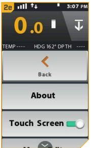
To toggle the Touch Screen "off", press the Touch Screen Touch Screen toggle will turn gray to indicate the Touch Screen is turned "off".
